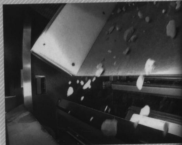
// Page 52 New freefall sorting installation for sorting waste materials
