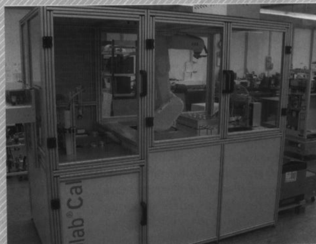
//Page 40 Clinker and cement reactivity in process control: automated isothermal heat flow calorimetry in lab automation
